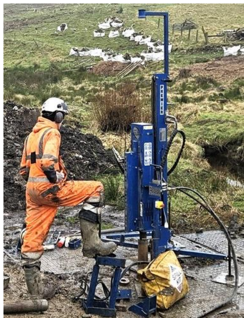
Figure 2: Modular style of rig used to carry out onsite borehole evaluation. Image credit: AOC Archaeology
