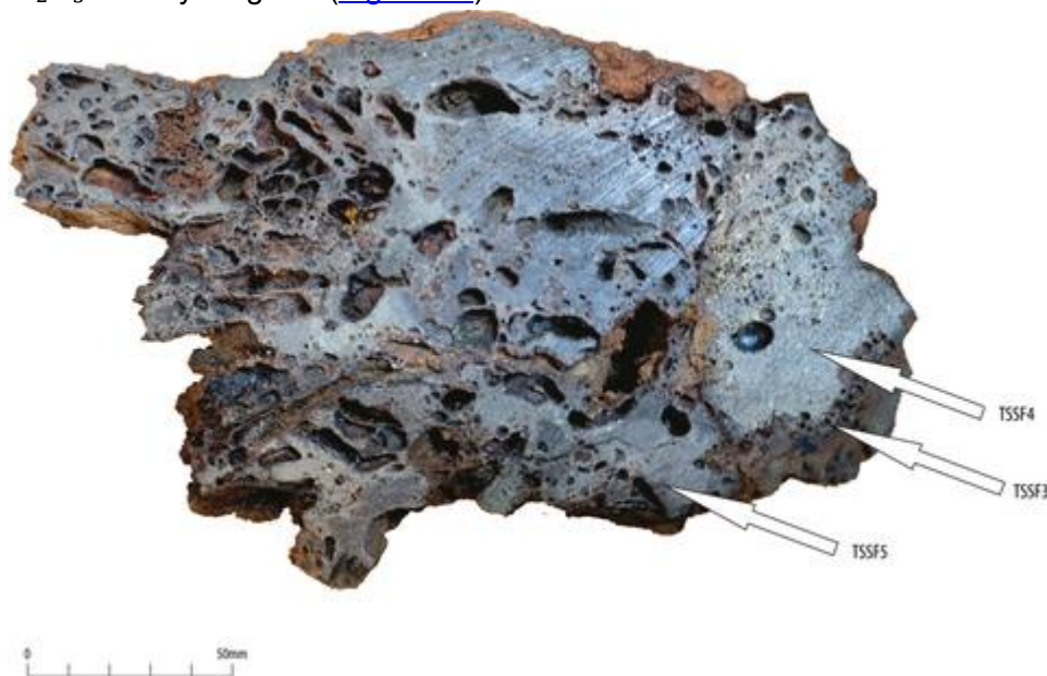
Figure 18: Details of locations of samples TSSF3-5 within a single large (2850g) slag block from ditch fill (074004). Sample TSSF5 is flow slag flowing away from the wall, sample TSSF3 is from a sliver of partially melted dark grey wall, and TSSF4 is part of the burr, or burr-like, zone of interaction between the slag and wall (Young 2025a , 72)
